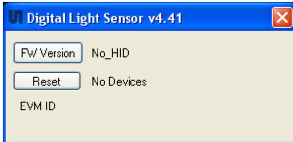
If “No Devices” appears, verify that the daughterboard is connected to the motherboard properly. If “No\_HID” appears, verify the USB cable is connected. A green LED on the motherboard indicates that the USB cable is connected and providing power to the system.
