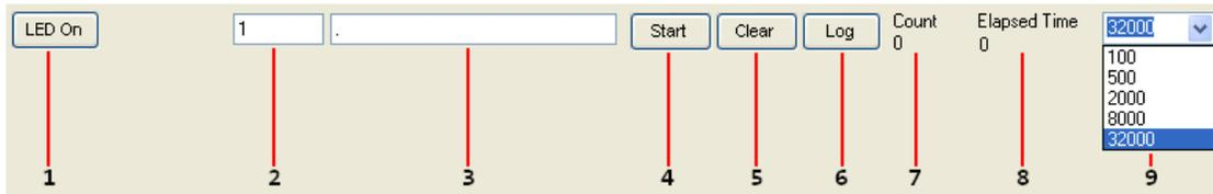
1. Toggles LED on the controller board.
