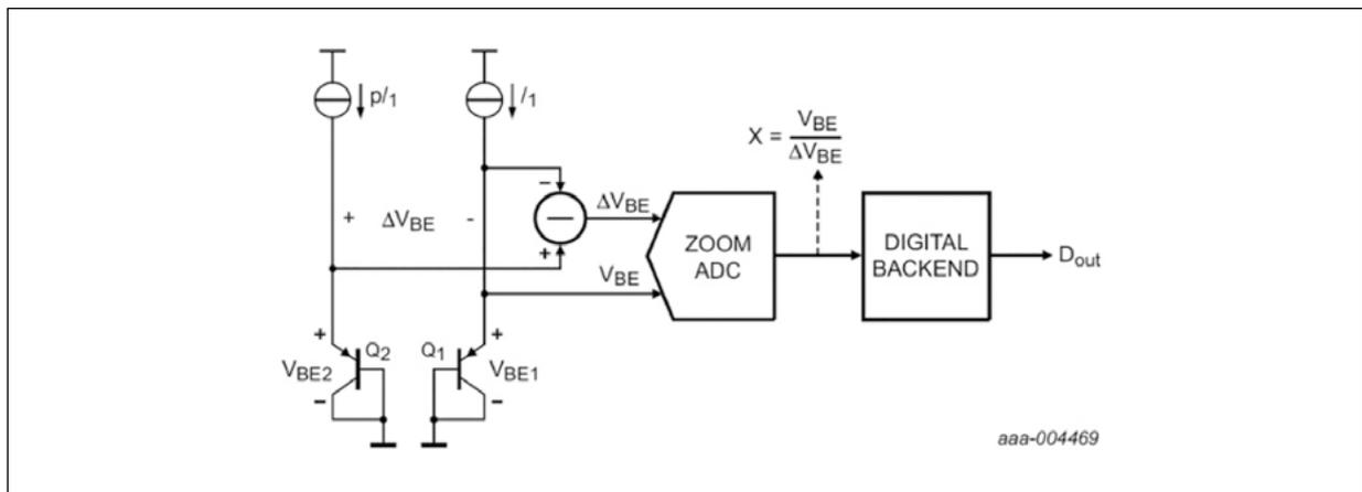
The temperature is measured using a high-precision (12 bits) zoom-ADC. The analog part is able to measure a strongly temperature dependent  $X = V_{BE} / \Delta V_{BE}$ . The  $X$  is found by first applying a coarse search (successive approximation), and then a sigma-delta in a limited range. The accuracy of the sensor is shown in Figure 12. The conversion time is shown in [Figure 9](#).
