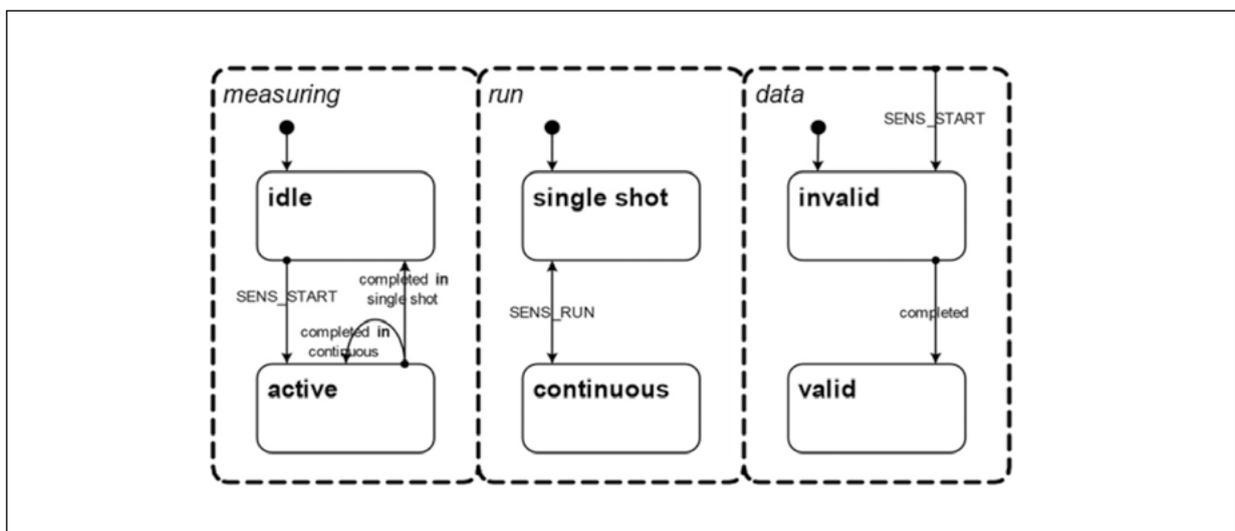
When in the *single shot* run mode, starting a measurement is under control of the master. By default a sensor is idle; it can be started by writing a 1 to the corresponding bit in SENS\_START. After a start, the sensor stops when the measurement is completed. Whether a sensor is idle or active measuring can be detected by reading SENS\_STAT. The measured values can be obtained via their respective readout registers (T\_VAL and H\_VAL). Writing to SENS\_STOP in single shot has no effect.
