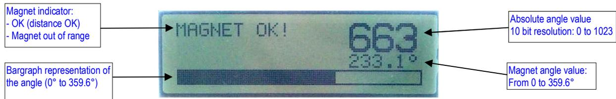
Figure 2: LCD display in standalone mode (9V battery or USB powered without GUI)
