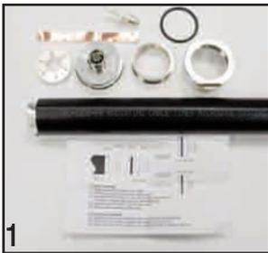
**Step 1:** Connector assembly parts for nuTRAC-1250FR (With modified collar and adhesive copper tape).
