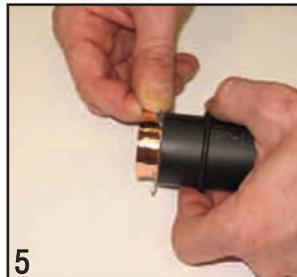
**Step 6:** Apply adhesive copper tape completely around the cable core shields. Both inner and outer shield will be in full contact with tape. Both drain wires will be outside the copper tape.
