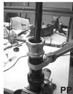
NOTE 1. Photo "YY" is an example of EX-13-3 Series Plug using Exd gland.
