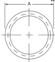
Used when open-back wiring is desired behind panelboards or within large junction boxes on which the basic barrel is mounted
