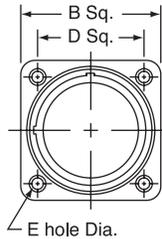
Drill hole in panel 1/64" larger than Dimension "H" for back mounting..
