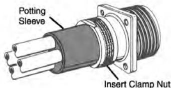
For use with insert clamp nut or panel board adapter to accept compound for sealing wire terminals. Potting sleeves are not for use with pressure-type contact units with insulator extension at back.
