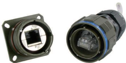
RJF TV allows you to use an Ethernet Class D / Cat. 5e connection for 10 BaseT, 100 BaseTx or 1000 BaseT networks in harsh environments. With the patented RJStop system you can use a standard RJ45 cordset in a **metallic** plug which will protect it from shocks, dust and fluids. **No hazardous on-field cabling and grounding!**
