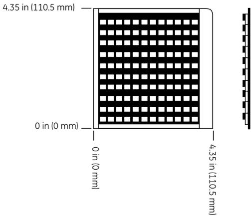
1. Sensors are shipped as 120 UP snapstrates that must be singulated by the customer.
