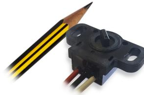
Despite its lightweight and miniature size of only 21mm., this hall effect sensor delivers high performance with up to 360° electrical angle (without dead zone), 12bit resolution, extended life and EMI & ESD protection.
