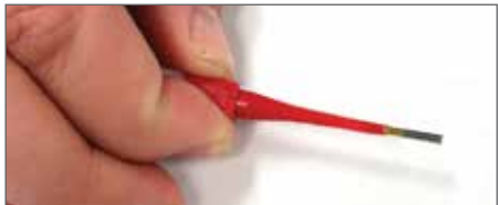
Plastic tool with contact in proper position.
