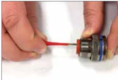
Plastic tool with contact in proper position.
