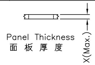
Screw L=5.0 For Panel Thickness Under 1.2mm
