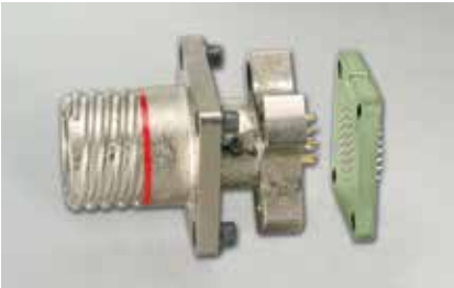
HEADERS PROVIDE EASY SEPARATION OF THE CONNECTOR FROM THE PC BOARD.
