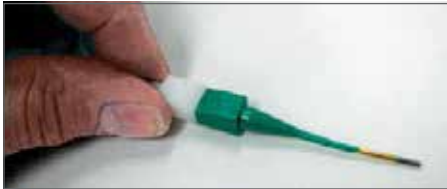
Plastic tool with contact in proper position.
