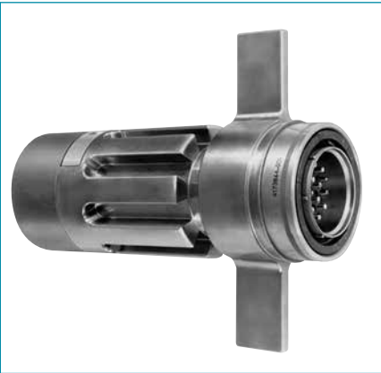
Special configuration Fail-Safe used on space telescope application. Lanyard is replaced by a swivel ring for remote disconnect and “wing arms” have been added for manual actuation accessibility by gloved astronauts.
