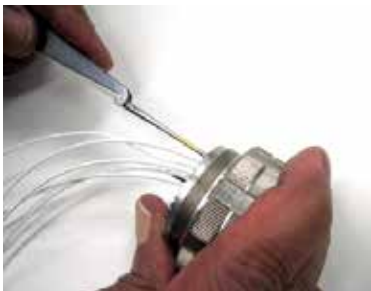
Removal of contacts with metal tool.
