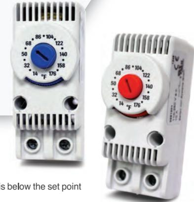
The Heating version (red dial, NC) has closed contacts when the temperature is below the set point value and opens with rising temperature.
