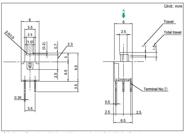
Only the configurations with the straight terminal are indicated in the dimensions.
