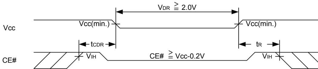
**Low V<sub>CC</sub> Data Retention Waveform (2)** (LB#, UB# controlled)
