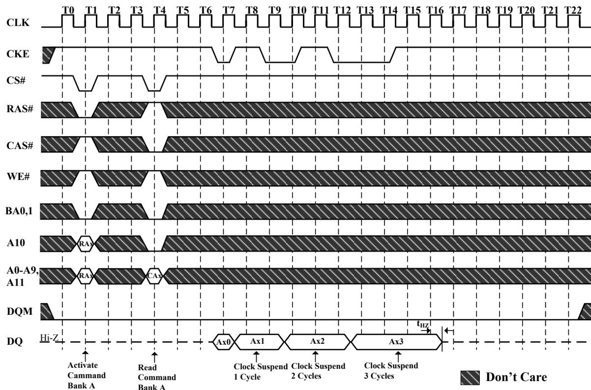
**Figure 25. Clock Suspension During Burst Write (Using CKE)**
