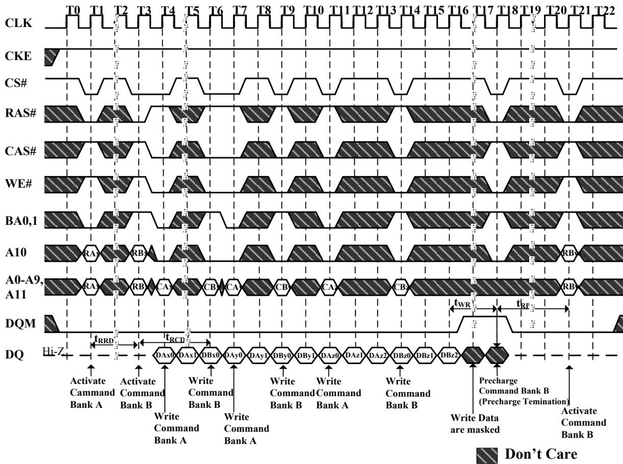
**Figure 42. Precharge Termination of a Burst**
