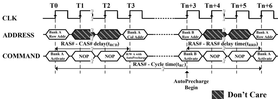
**Figure 3. BankActivate Command Cycle (Burst Length = n)**
