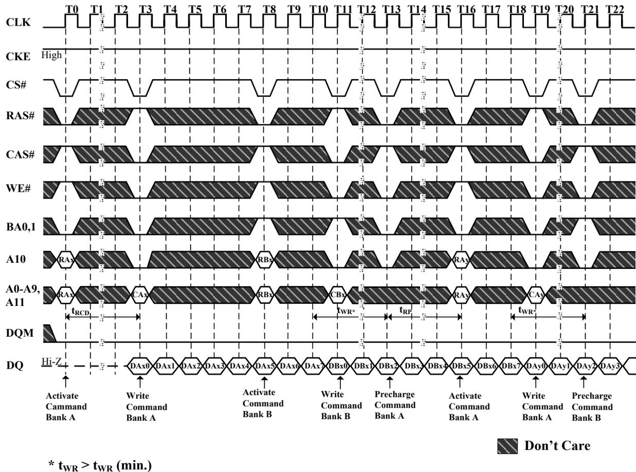
**Figure 31.1. Read and Write Cycle (Burst Length=4, CAS# Latency=2)**
