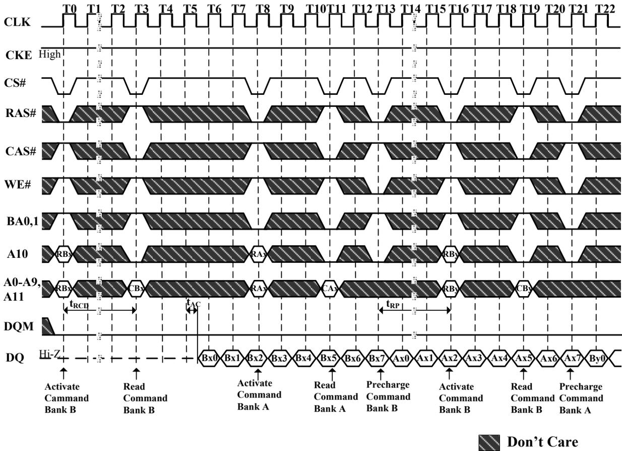
**Figure 30. Random Row Write (Interleaving Banks)**
