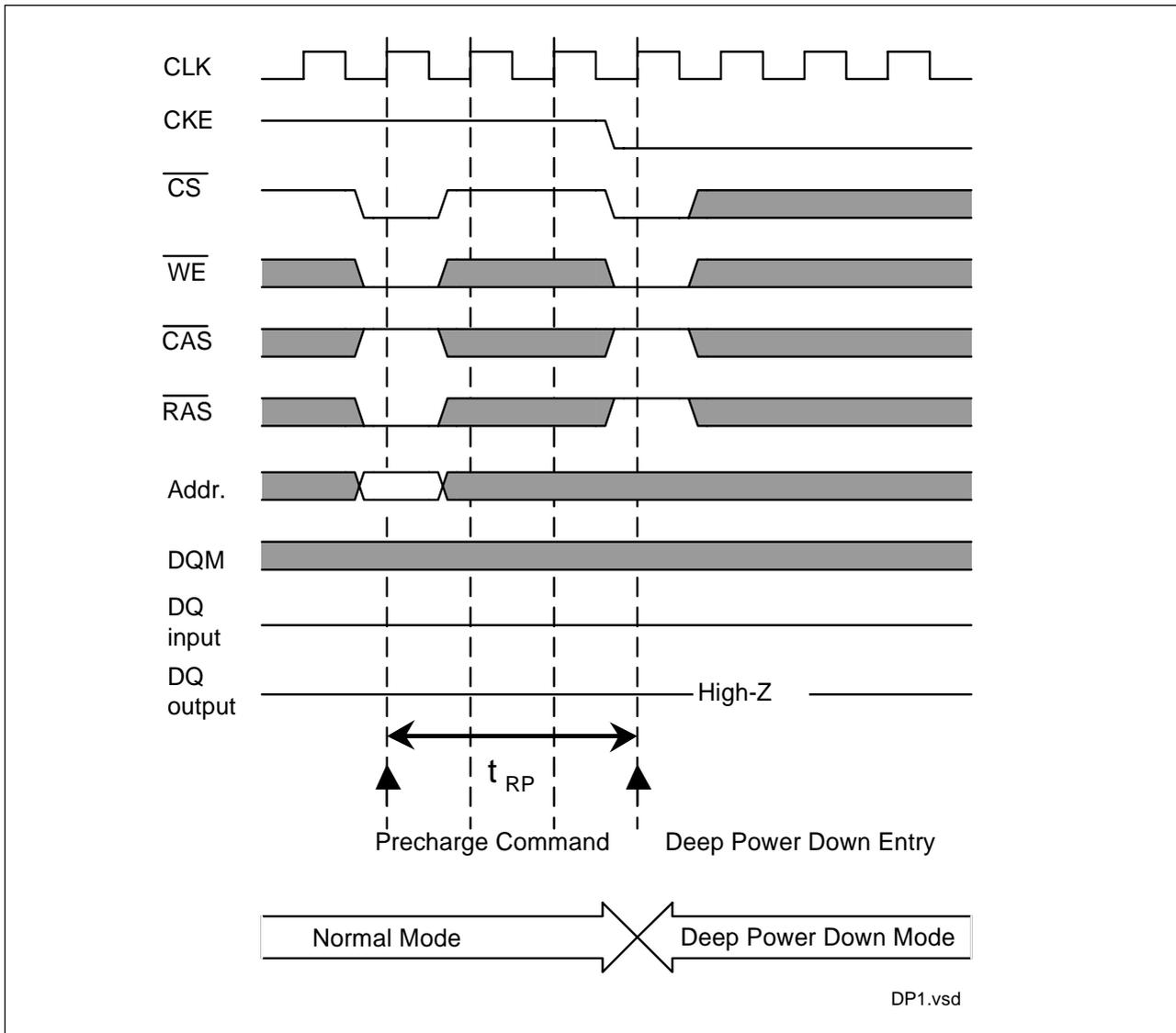
The deep power down mode has to be maintained for a minimum of 100 $\mu$ s.
