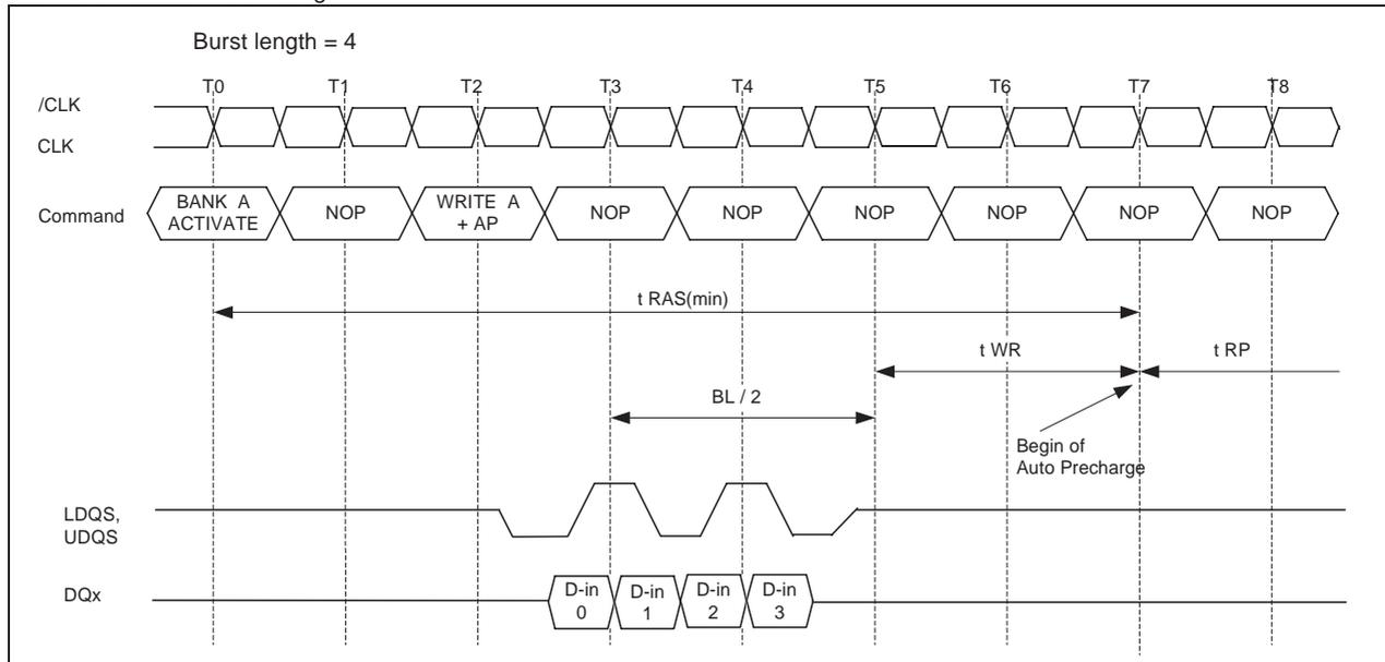
Note:  $t_{WR}$  starts at the first rising edge of clock after the last valid edge of the 4 DQSx.
