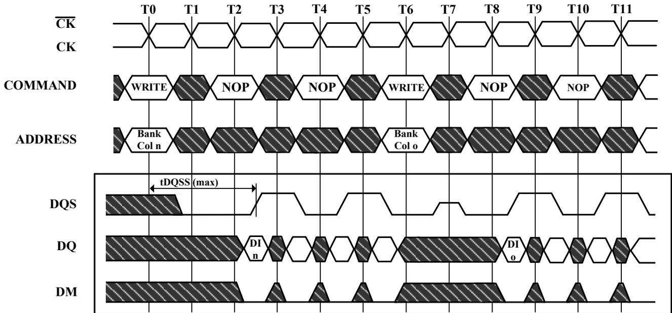
DI<sub>n</sub>, etc. = Data In for column n, etc.
