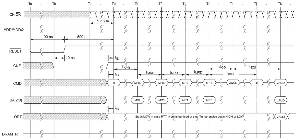
1) From time point 'Td' until 'Tk', NOP or DES commands must be applied between MRS and ZQCL commands
