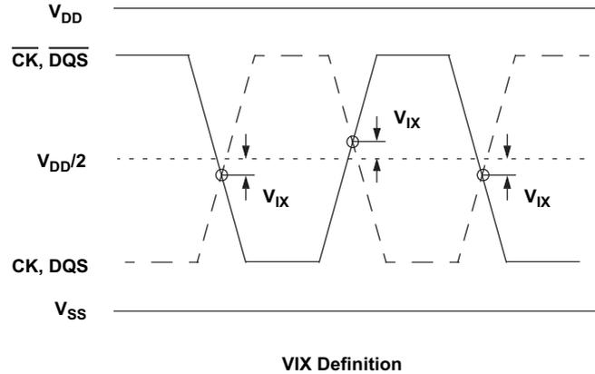
**Cross point voltage for differential input signals ( CK, DQS ): 1.35V**
