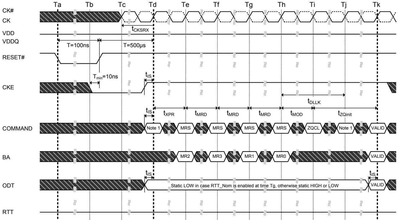
NOTE 1. From time point "Td" until "Tk" NOP or DES commands must be applied between MRS and ZQCL commands.
