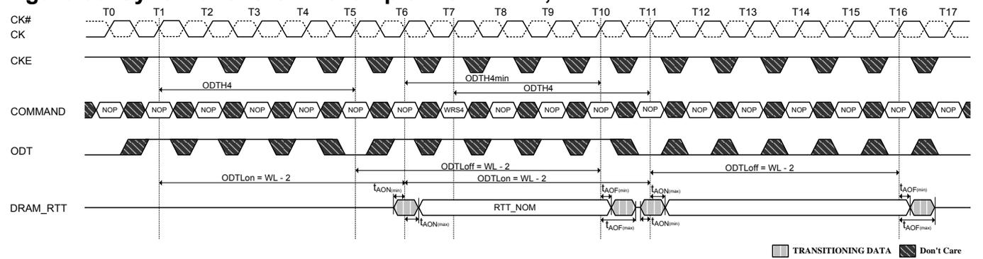
**Figure 67. Dynamic ODT Behavior with ODT being asseted before and after the write**
