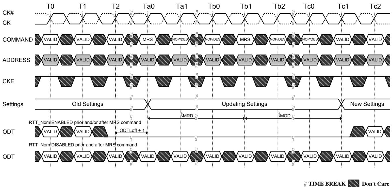
The MRS command to Non-MRS command delay,  $t_{MOD}$ , is required for the DRAM to update the features except DLL reset, and is the minimum time required from an MRS command to a non-MRS command excluding NOP and DES shown in Figure 7.
