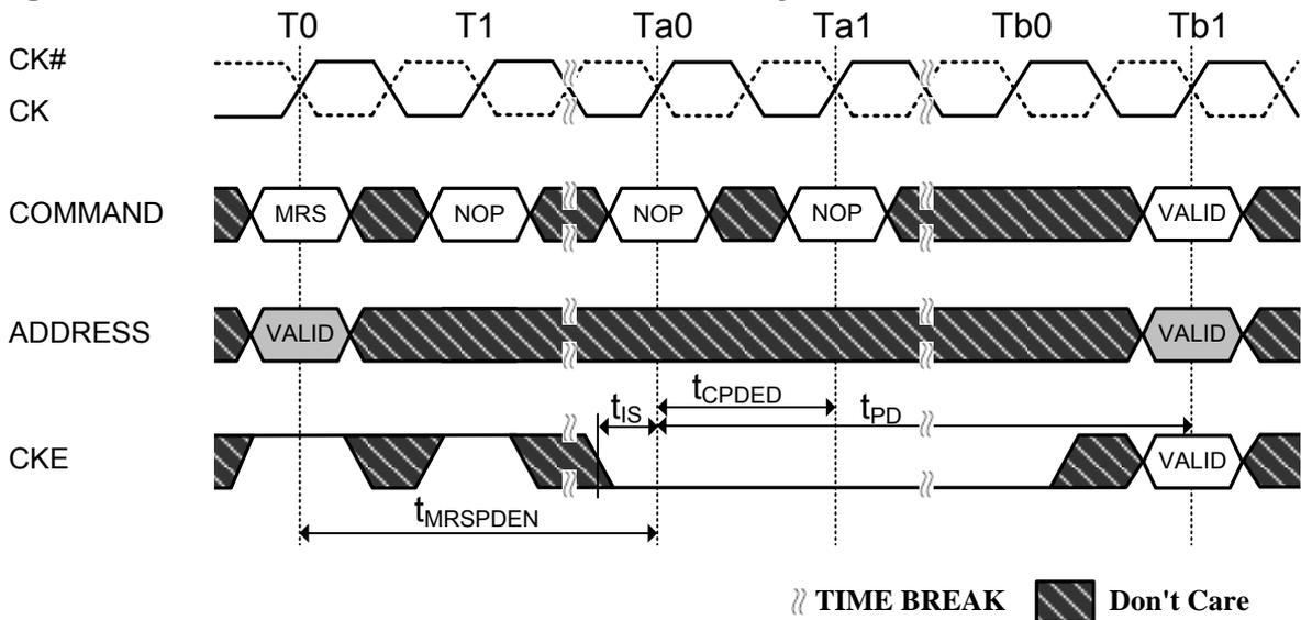
**Figure 65. Synchronous ODT Timing Example**
