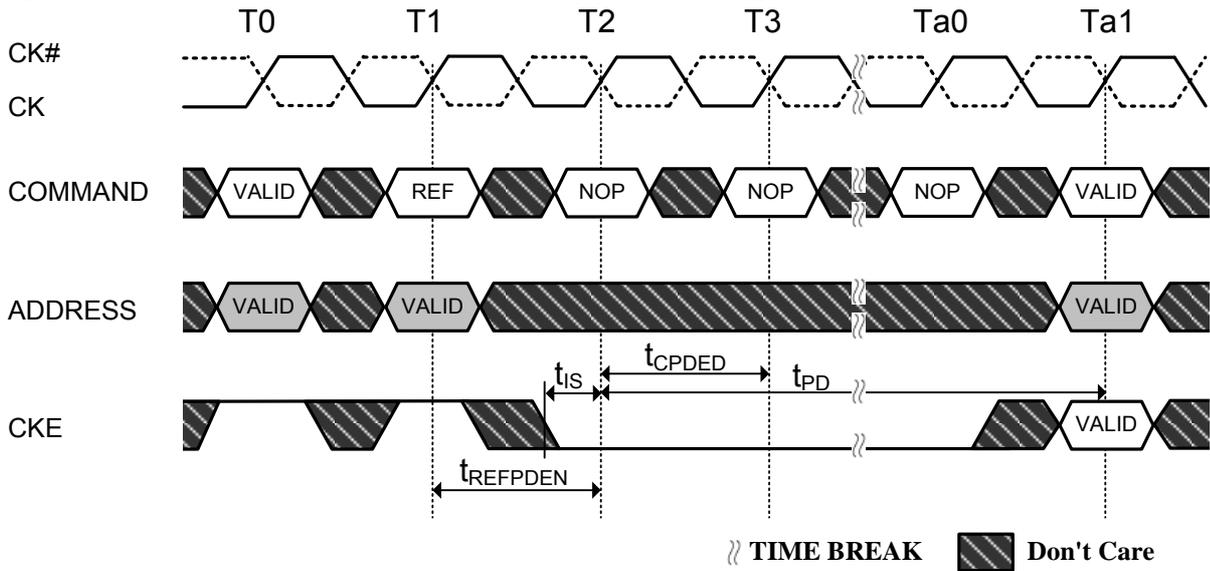
**Figure 62. Active Command to Power-Down Entry**
