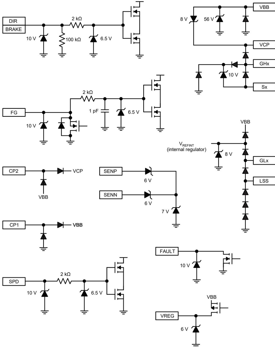
Figure 8: Terminal Diagrams
