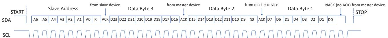
Figure 7: Read from an I<sup>2</sup>C register
