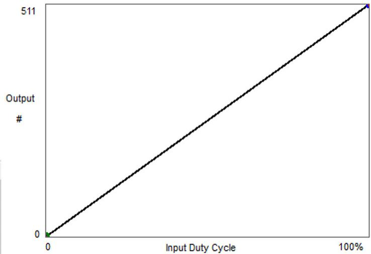
*Example 1:* These screenshots are taken from the A89307 application—white boxes are the entered values. This is the most trivial example, where input = output. This is the curve that is used when the transformer is disabled. Because 511 is the input value in the second address, the 30 following addresses are ignored.
