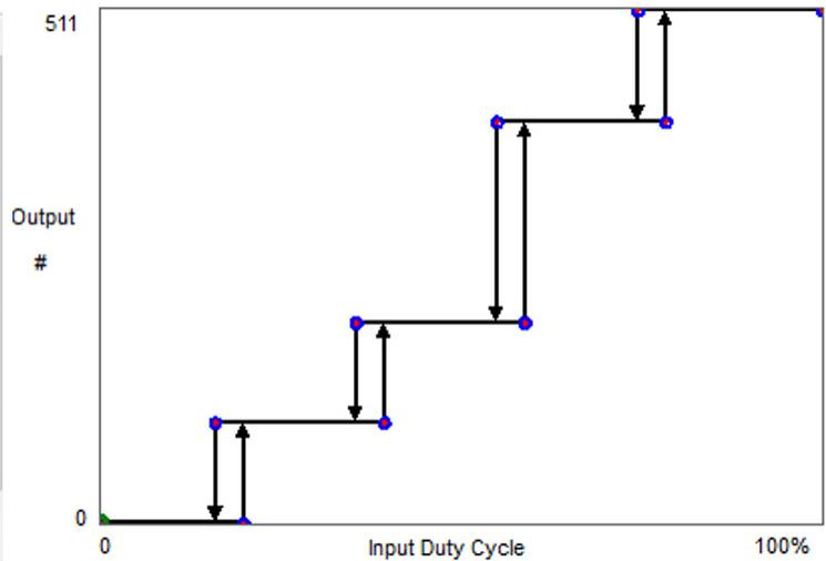
Example 3: Hysteresis can be implemented by setting the input value of an address lower than the input value in the previous address. In this example, as the input demand is rising, the output demand will jump to next higher level at the vertical lines on the right of each transition. When the input demand is falling, the output demand will drop to next lower level following the vertical lines on the left of each transition. This prevents output jitter when the input is around a boundary.
