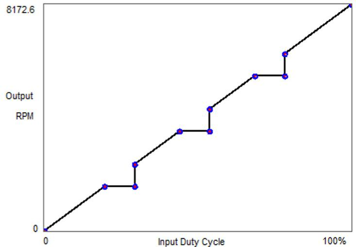
*Example 2:* In this example, the control loop is set to closed-loop speed, and so the resulting rpm is shown in the last column of the table where the curve is defined. This curve is designed to avoid this motor’s resonant frequency at 2000 rpm, and its harmonics at 4000 rpm and 6000 rpm.
