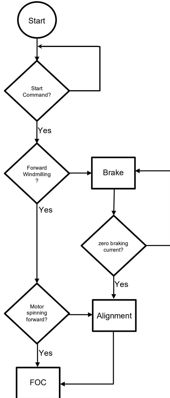
**Rotor Alignment:** When the A89307 is commanded to spin the motor, the controller will execute motor rotor alignment to ensure the rotor is parked at a known position. There are four different modes to achieve rotor alignment or detection.
