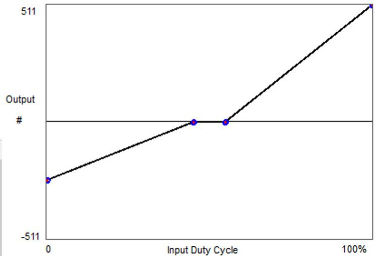
*Example 5:* The curve can be set to control bi-directional operation as well. When the bidirectional option is selected, the output value 511 is still the highest output in one direction, but the output value 255 will stop the motor, and the output value 0 is the highest output in the reverse direction. Here, the motor will run at half speed reverse when input demand is 0, will stop when the input is between 230 and 280, and will run at full speed forward when the input is 511.
