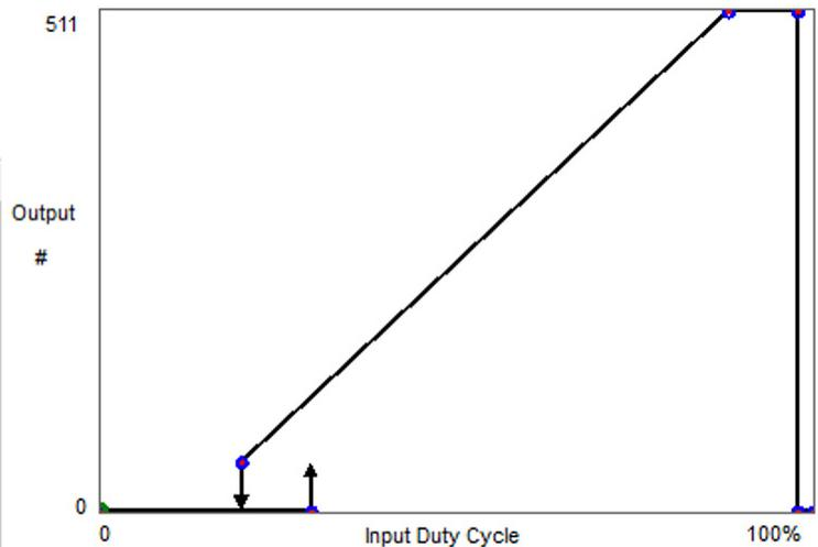
Example 4: In this example, the motor won't turn on until the input is about 30% and will turn off when the output falls below about 20%. The output will be at maximum when the input is between about 88% to 98%, and the motor will stop when the input is > 98%.
