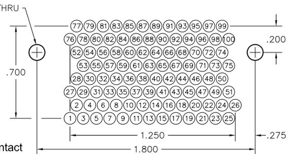
\* For pin (plug) connectors, the contact numbers are reversed left to right.
