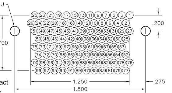
\* For pin (plug) connectors, the contact numbers are reversed left to right.
