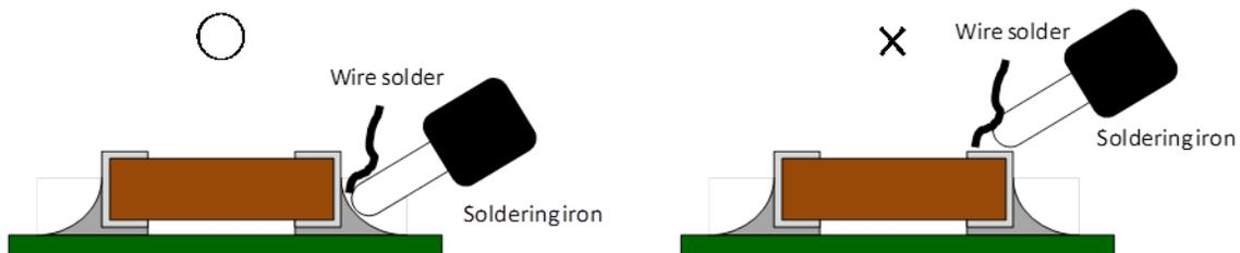
Fig 3 Correct handling method of soldering iron
