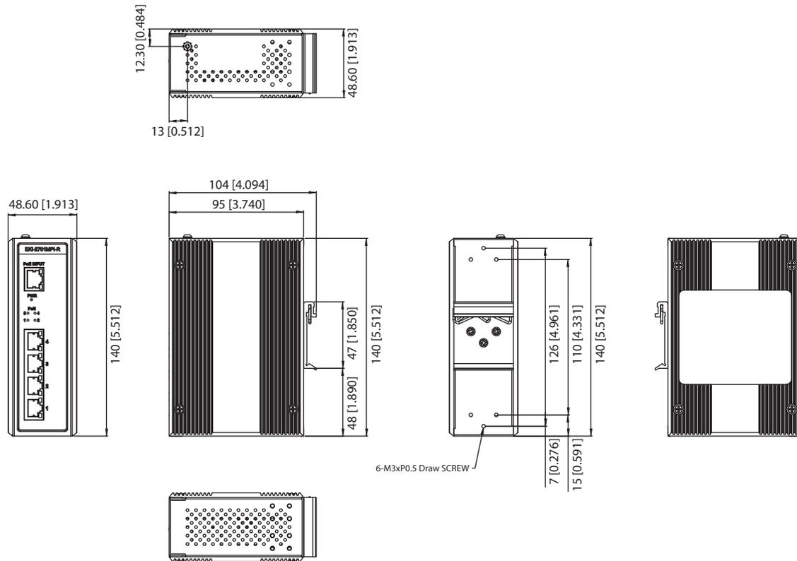
**Panel Cut-out Dimensions (W x H x D): 48.6 x 140 x 95 mm (1.91" x 5.51" x 3.74")**
