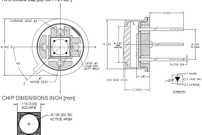
>Soldering Conditions: 260°C 1/16 inch away from case for 3 seconds max.
