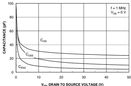
Figure 8. Capacitance Characteristics.
