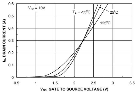
Figure 5. Transfer Characteristics.
