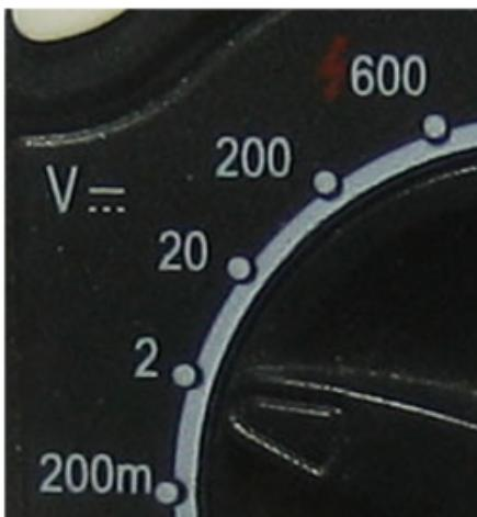
For this example, it's best to test with the output from the breakout connected to a multimeter in DC voltage mode. DC voltage mode is labeled with a V and two lines, one dashed and one solid. [For information on using a multimeter, check out this guide.](#) (<https://adafru.it/192A>)
