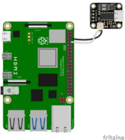
Pi GND to breakout JST SH GND (black wire)
