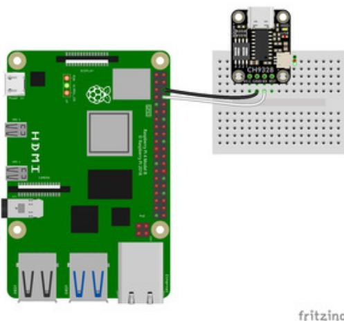
Pi GND to breakout GND (black wire)
