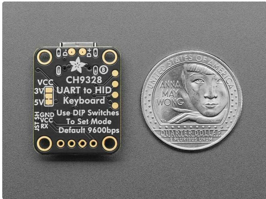
You can configure the 'Mode' using the 4 on-board switches, do that before powering it up:
