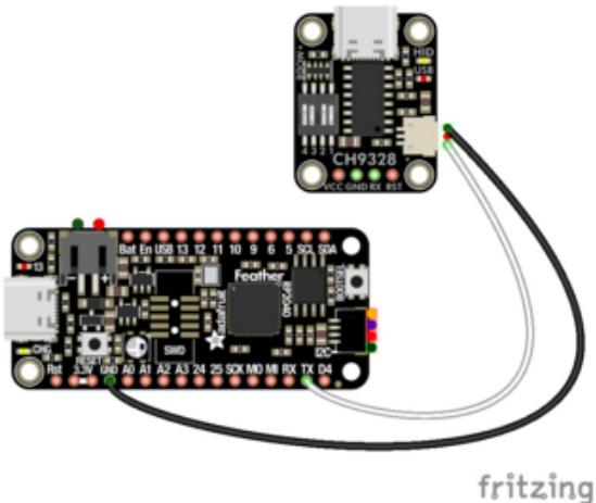
**Board GND to breakout JST SH GND
