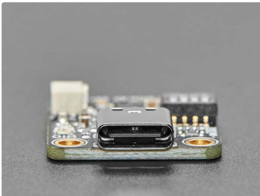
The [CH9328](https://adafru.it/1a2F) (<https://adafru.it/1a2F>) is a funky chip that is basically a programmed microcontroller that enumerates as an every-day HID keyboard and can convert ASCII or 8-byte raw reports, read over a standard serial port UART, into keypresses. So, you can emulate a keyboard even if your chip doesn't have native USB! You do need a hardware or software serial port: some way to generate 9600 baud 3V-logic signal that the CH9328 can read.
