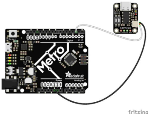
Board GND to breakout JST SH GND
