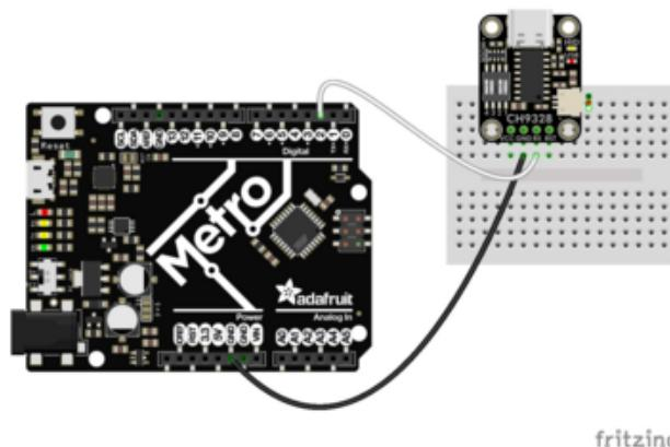
Board GND to breakout GND (black wire)
