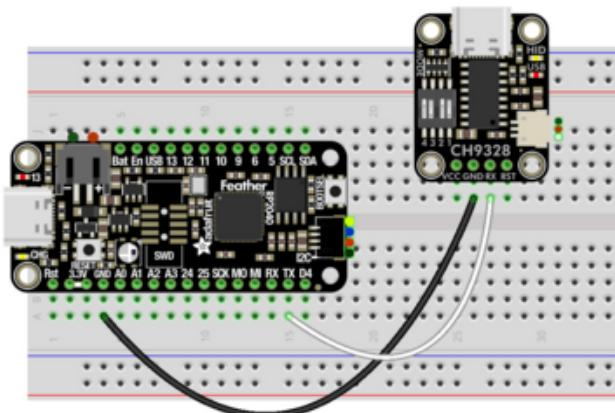
**Board GND to breakout GND (black wire)**
