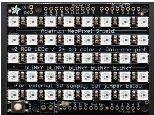
By default, the LEDs are powered from the Arduino's 5V pin. As long as you aren't lighting up all the pixels at full brightness that should be fine. Or power the shield with an external power supply by soldering the included terminal block.
