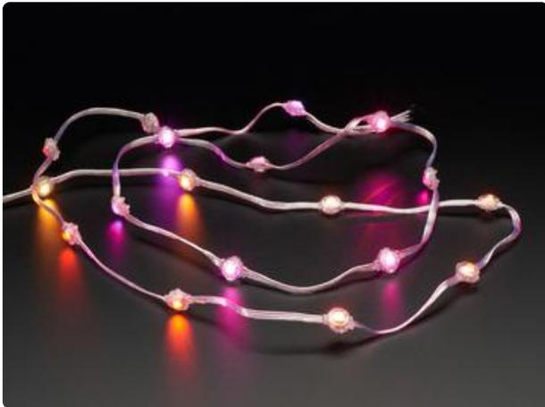
Like NeoPixel strips, these “strands” are flexible and can be wrapped around things. The pixels are spaced further apart (2 or 4 inches) with each pixel is sealed in its own tiny plastic capsule, making them weatherproof (but not rated for continuous submersion). There are 20 pixels in a strand.
