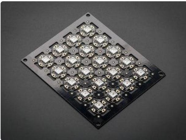
The original Adafruit NeoPixel form factor! Flora RGB Smart NeoPixels were designed for wearable projects using conductive thread, but can also be soldered normally with wires. These are available in two formats:
