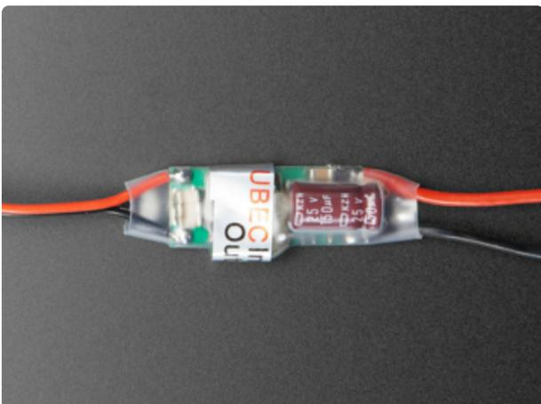
A [buck converter \(https://adafru.it/efD\)](https://adafru.it/efD) can efficiently step a higher DC voltage down to 5V for NeoPixels and microcontrollers ... for example if you have a 12V power source, like a car battery.
