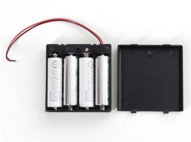
Four nickel-metal hydride (NiMH) rechargeable cells can similarly be used in a [4-cell battery holder \(http://adafru.it/830\)](http://adafru.it/830) to provide 4.8 Volts.
