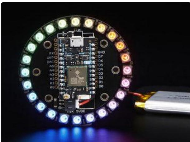
Previously mentioned on the “Rings” page, but for posterity: this [24-pixel RGB ring \(http://adafru.it/2268\)](http://adafru.it/2268) is specifically designed for the Particle (formerly Spark) Photon development board.
