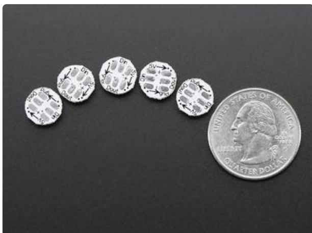
NeoPixel Mini Button PCBs are the smallest ready-to-use NeoPixel format — each on its own tiny board with an input resistor and decoupling capacitor.
