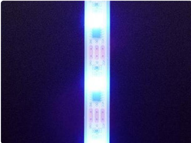
A single-color ultraviolet variant of NeoPixel strip is available for special applications, currently one pixel density and backing color:
