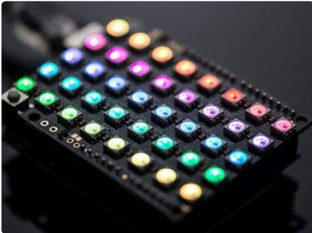
This 5x8 [NeoPixel Shield for Arduino](http://adafru.it/1430) (<http://adafru.it/1430>) fits neatly atop an Arduino Uno or compatible boards (5V logic recommended). Like many of our NeoPixel products, they're available in RGB and various RGBW pixel types:
