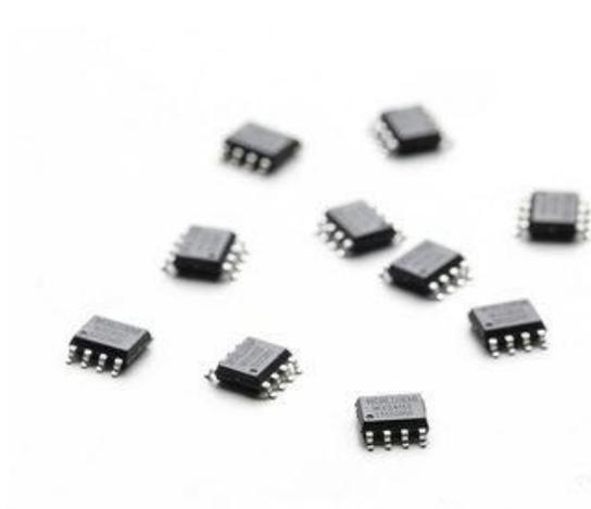
The NeoPixel driver logic is available separately (<http://adafru.it/1378>) from the LEDs, allowing power-users to create extremely customized designs...perhaps using other LED colors, or combined with power MOSFETs (<http://adafru.it/355>) to control high-current LEDs or “analog” RGB LED strips (<https://adafru.it/ICy>) using the NeoPixel protocol.
