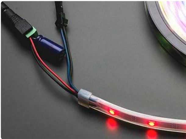
Before connecting a NeoPixel strip to ANY source of power, a large capacitor (500–1000  $\mu\text{F}$  at 6.3 Volts or higher) across the + and – terminals provides a small power reservoir for abrupt changes in brightness that the power source might not otherwise handle — a common source of NeoPixel “glitching.”
