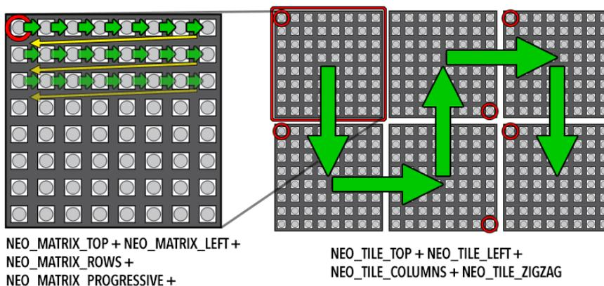
Tiles don't need to be square! The above is just one possible layout. The display shown at the top of this page is three 10x8 tiles assembled from NeoPixel strip.
