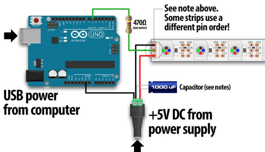
When connecting NeoPixels to any LIVE power source or microcontroller, ALWAYS CONNECT GROUND (-) BEFORE ANYTHING ELSE. Conversely, disconnect ground last when separating.
