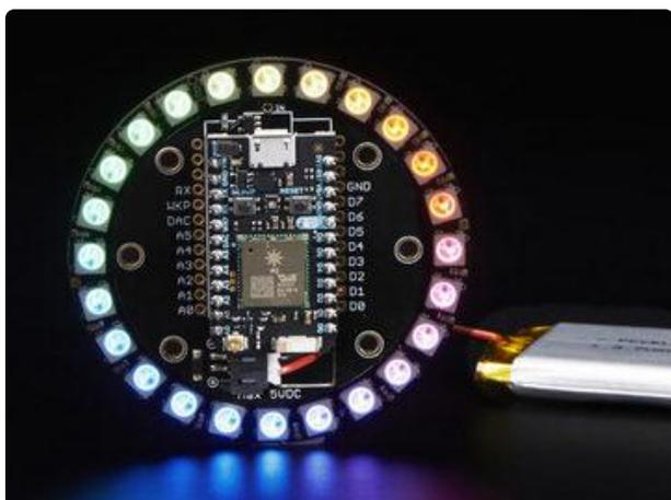
There's also a [24-pixel RGB ring \(http://adafru.it/2268\)](http://adafru.it/2268) specifically designed for the Particle (formerly Spark) Photon development board.
