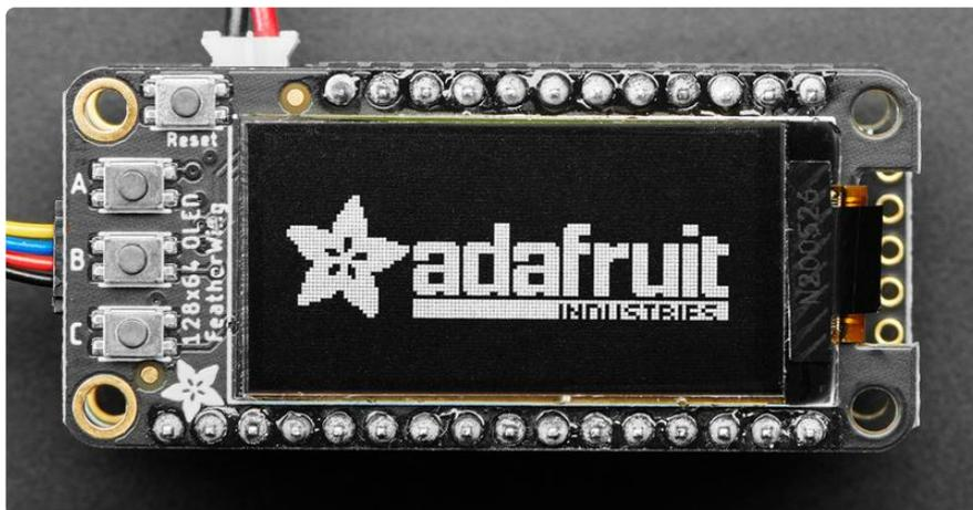
It's easy to use the Adafruit 128x64 OLED FeatherWing with CircuitPython and the [Adafruit CircuitPython DisplayIO SH1107 \(https://adafru.it/OaL\)](https://adafru.it/OaL) module. This module allows you to easily write CircuitPython code to control the display.
