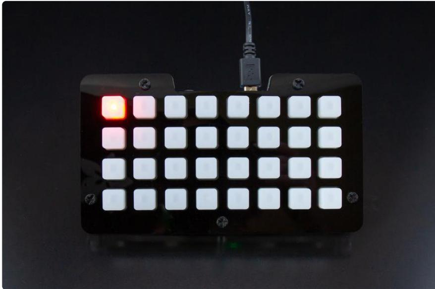
The TrellisM4 library has the ability to specify four different orientations in 90 degree increments by setting `rotation` in the setup line equal to: 0, 90, 180, or 270. This allows you to rotate your board with ease to the position that works best for your project, without requiring complicated code to compensate. We do that for you! The coordinates of the buttons change with the rotation, so `(0, 0)` is always top-left. Let's look at some examples.
