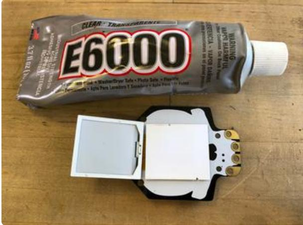
Use a toothpick or skewer to place small dabs of the glue around the perimeter of the backlight.
