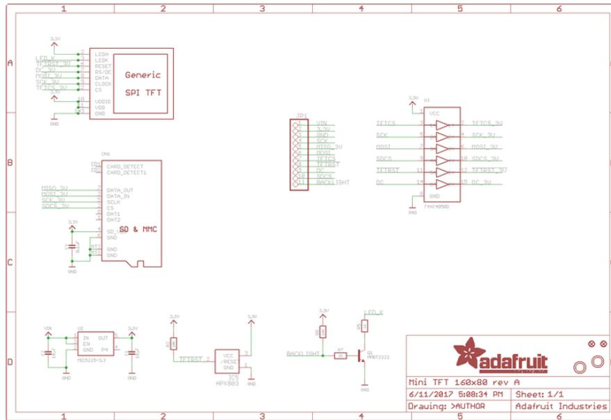
For the level shifter we use the [CD74HC4050](https://adafru.it/CgA) (<https://adafru.it/CgA>) which has a typical propagation delay of  $\sim 10$ ns
