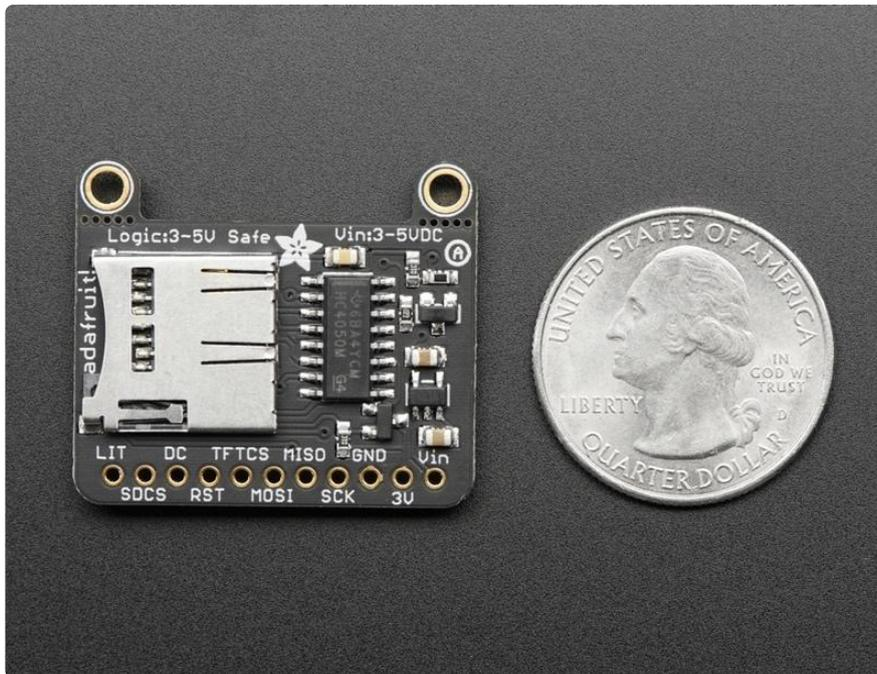
The breakout has the TFT display soldered on (it uses a delicate flex-circuit connector) as well as a ultra-low-dropout 3.3V regulator and a 3/5V level shifter so you can use it with 3.3V or 5V power and logic. We also had a little space so we placed a microSD card holder so you can easily load full color bitmaps from a FAT16/ FAT32 formatted microSD card. The microSD card is not included, [but you can pick one up here \(http://adafru.it/102\)](http://adafru.it/102).
