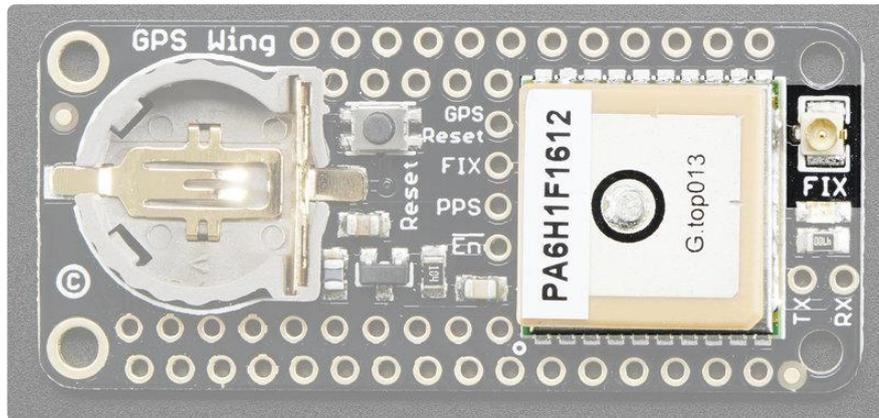
All Ultimate GPS modules have a built in patch antenna - this antenna provides -165 dBm sensitivity and is perfect for many projects. However, if you want to place your project in a box, it might not be possible to have the antenna pointing up, or it might be in a metal shield, or you may need more sensitivity. In these cases, [you may want to use an external active antenna. \(http://adafru.it/960\)](http://adafru.it/960)
