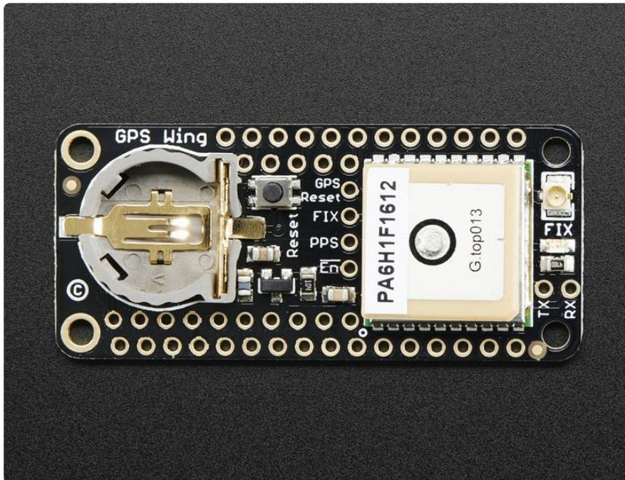
Give your Feather a sense of place, with an Ultimate GPS FeatherWing. This FeatherWing plugs right into your Feather board and gives it a precise, sensitive, and low power GPS module for location identification anywhere in the world. As a bonus, the GPS can also keep track of time once it is synced with the satellites.
