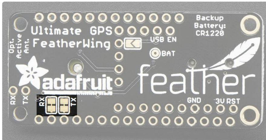
And then wire your desired pins to the RX and TX breakouts right next to the FIX LED
