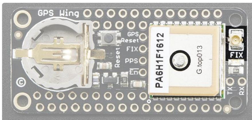
You have two options for an antenna. The GPS module has an antenna on it already, that's the square tan ceramic thing on the left side. If you plug an active GPS antenna into the uFL connector on the very right, the module will automatically switch over to the external antenna.
