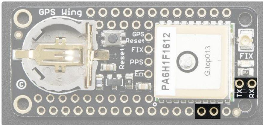
The GPS module, like pretty much all GPS's, communicates over UART serial. It sends ASCII NMEA sentences from the GPS TX pin to the microcontroller RX pin and can be controlled to change its data output from the GPS RX pin. Logic level is 3.3V for both.
