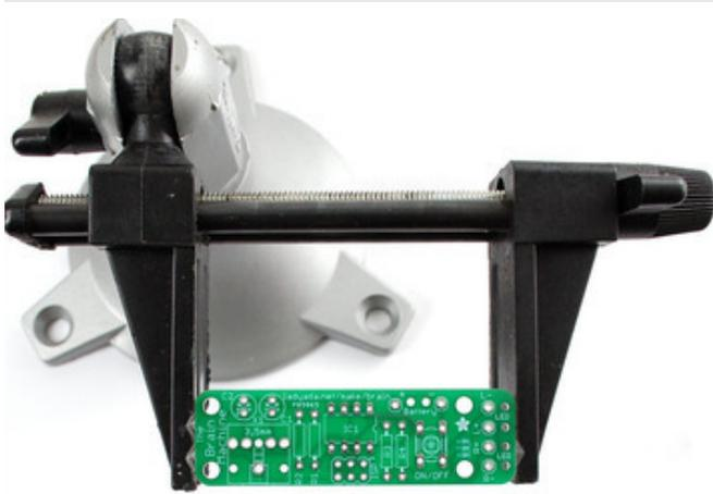
Place the PCB in a vise (if you have one), and turn on the soldering iron. [Make sure you have all the tools you'll need to assemble the kit.](https://adafru.it/c1y) (<https://adafru.it/c1y>)
