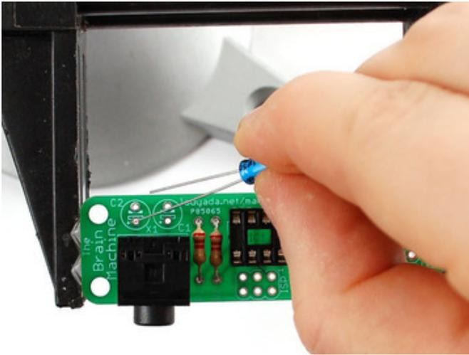
Next are the two electrolytic capacitors **C1** and **C2**. These help smooth the output of the microcontroller audio generation to make it less squeaky.
