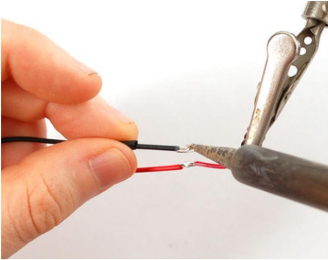
Next solder the black wire to the brown wire. Make sure the heat shrink is on the battery pack wires but out of the way so you don't accidentally heat them up before it's time.
