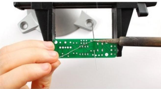
Solder joints should be smooth and shiny and fill the entire pad, wicking up to the lead. you shouldn't be able to wiggle the wire and have it move in the hole.
