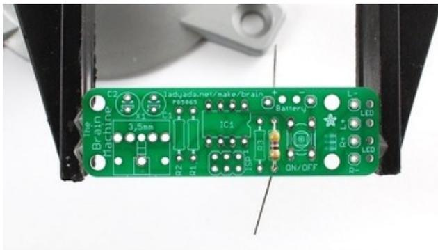
The first part we will place is the resistor **R4** - this is a small oval tan thing with two wires (leads) and color stripes. The stripes are yellow violet black which indicates a 47 ohm resistor. This resistor is used to set the brightness of the lightbulbs (LED) for the right eye. A smaller resistor (less resistance) would make the LED brighter. A larger resistor would make the LED dimmer.
