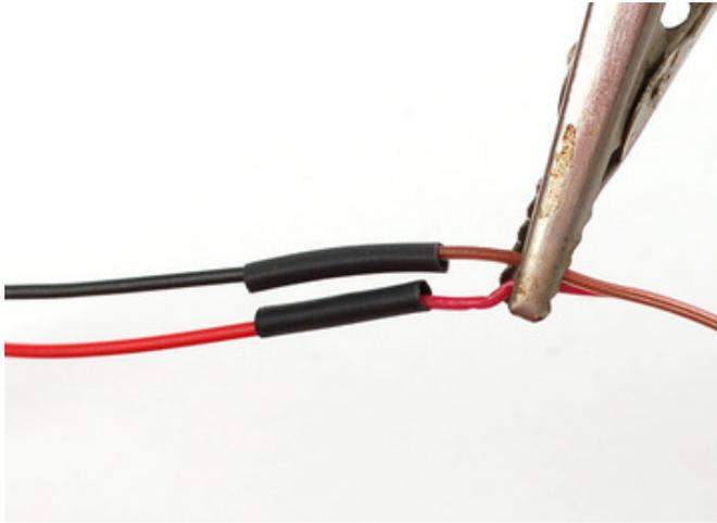
Once the wires are soldered, slip the heatshrink so that it covers the soldered joints.
