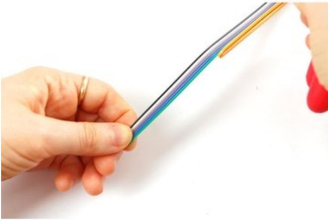
Use the clip and tear technique to pull off three strips of two wires each. One is red/brown, another orange/yellow and the last pair green/blue.
