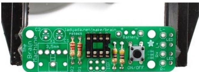
The socket has a little **U** in one end. The **U** should match the **U** in the silkscreen image printed on the PCB. In this photo the **U** is on the right.
