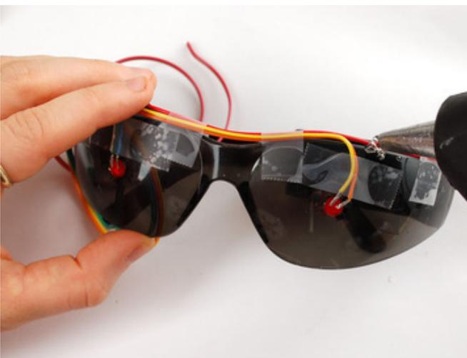
As in the photo, make sure that the arms of the glasses are folded, and use your adhesive of choice to glue the wires to the top of the glasses. The tape will keep the wires in place while the glue hardens.
