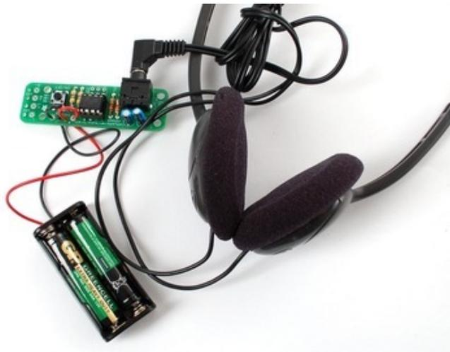
(Optional: if you think you would like to re-program your Brain Machine's microcontroller, solder in the 2x3 pin socket into the 6 pins marked "ISP" on the PCB. Be sure to place the short leads into the PCB.)
