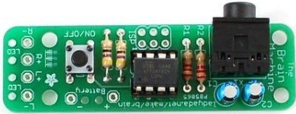
Now we can place the microcontroller chip. This chip holds the brain machine program and is 'burned in' here at the Adafruit factory.
