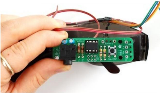
Start with the two power wires (red/brown). Place the PCB on the arm, maybe use tape to hold it in place, and cut the red/brown wire pair so that you have plenty of wire to solder it to the **Battery** terminals (but not so much it's a big mess) -- about 2" extra length is sufficient. (I cut it a little shorter than necessary, give yourself plenty of space!)
