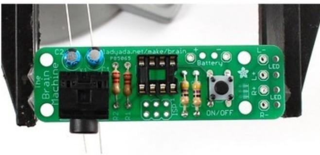
Solder in the capacitors and clip the long wires.
