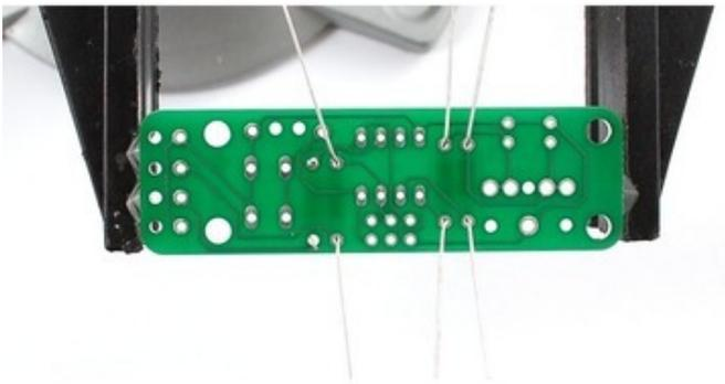
Then place both **R1** and **R2** they are both 2.2K resistors (red-red-red). These resistors set the loudness of the earphones for either ear. Using a larger resistor (more resistance) would make the volume quieter. Using a smaller resistor would make the volume louder.
