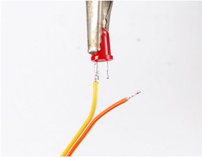
Clip the remaining LED wire and solder the orange wire to it.
