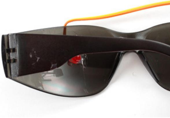
Squeeze a big blob of hot glue on to the left arm of the glasses and stick the battery pack on, making sure that the wires from the battery pack are facing the front of the glasses.
