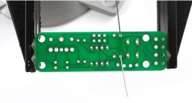
Resistors are **non-polar** which means they don't have a direction: you don't have to worry about putting it in 'backwards' because they work the same either way.
