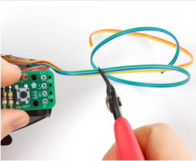
Cut the Orange/Yellow and Green/Blue wires so that there is plenty of slack for them to reach the LED solder holes on the right edge of the PCB. Be sure to have enough wire so that you can fold the arms of the glasses.
