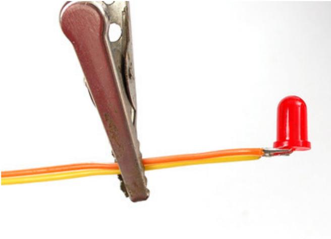
Finally, bend both LEDs (gently and only once) so they are at right angles to the wire. It doesn't matter which way they are bent. The easiest way to do this is to hold the LED in one hand and use a finger to bend the wires.
