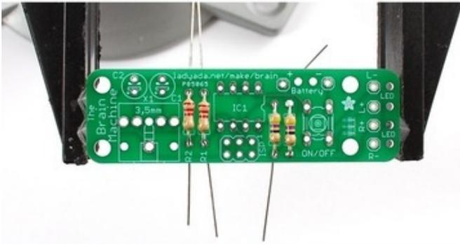
There are another 3 resistors and we'll finish them all up. Place resistor **R3** (another 47 ohm yellow-violet-black) resistor right next to **R4**. This is the resistor that sets the brightness for the other eye's LED.
