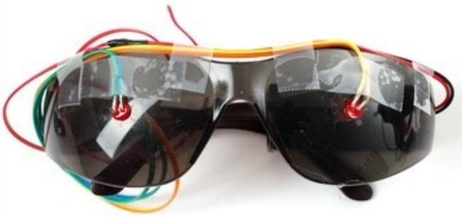
Use tape to attach the red/brown, orange/yellow and blue/green wires to the top edge of the glasses so they run together.
