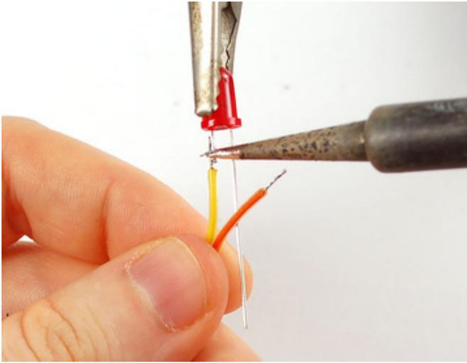
Because there is already solder on the LED and wire, you should be able to hold the yellow wire to the short lead and heat it up with the iron and they'll melt together and hold.
