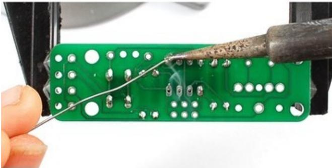
You might want to start by soldering two corner pins. This keeps the socket on straight while you do the rest.
