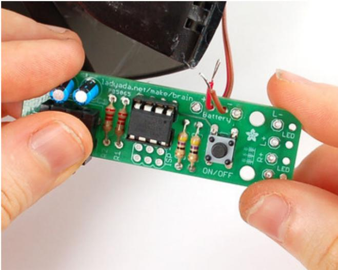
Cut, trim, split, strip and tin the wires. Then slide the **Red** wire through the hole marked + (positive, plus) and the **Brown** wire through the hole marked - (negative, minus).
