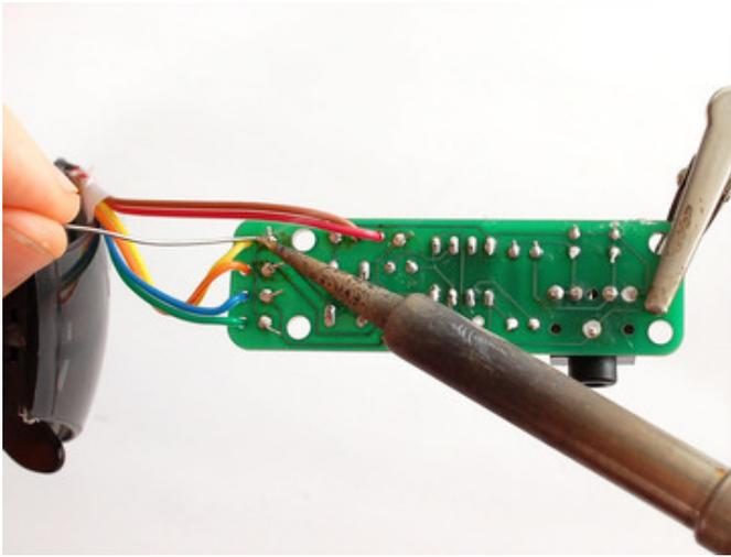
After you've tested the board, remove the AAA batteries and solder in the four wires.
