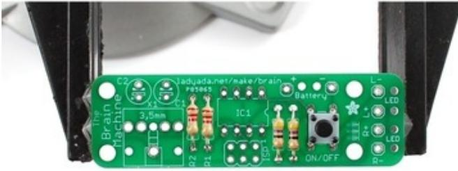
Next is the tactile button that is used to tell the microchip in the kit to turn on and off. The button is also nonpolar (it's just a mechanical switch) so you cant put it in 'backwards' It should snap into place right next to the **ON/OFF** silkscreen label on the PCB.
