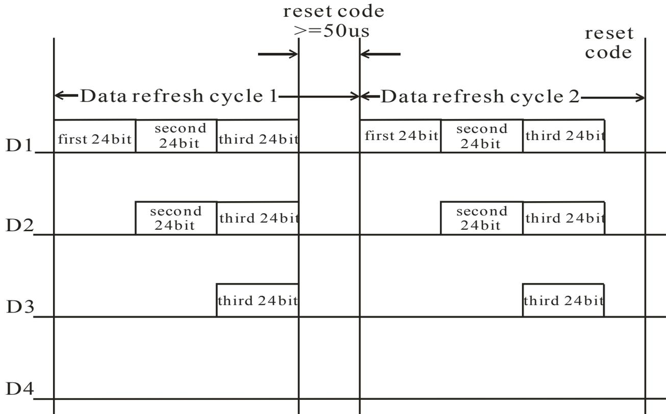
Note: The data of D1 is send by MCU, and D2, D3, D4 through pixel internal reshaping amplification to transmit.
