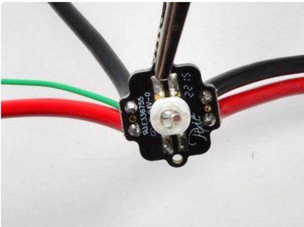
You can use a thinner wire for data, in this case we have a ~22AWG data line. It's soldered onto the out pin here
