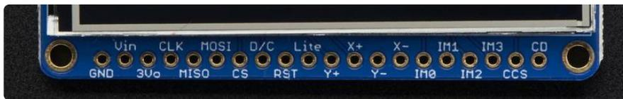
Don't forget, we're using the SPI interface side of the PCB!
