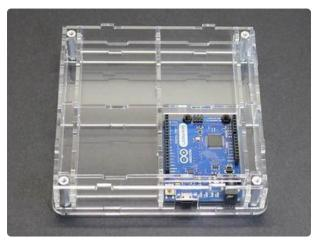
The four side pieces are almost identical...except for one which has a notch for the Arduino's USB port. Install this side first. Align the bottom tabs with the slots in the base and tilt it up into place. If the USB port is covered, you've got it backwards — turn it around and try again.
