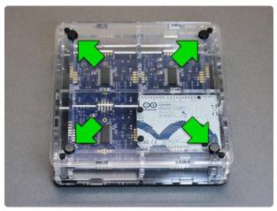
Turn the whole thing over and peel-andstick the four rubber feet near the corners.
