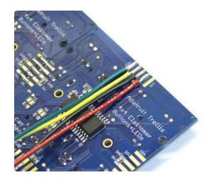
Try pointing the wires "inward" rather than off the edge of the board. This makes it easier to fit in the case.
