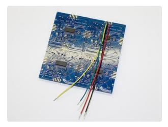
Looking at the back of the tiled Trellis boards...with the text upright, in the normal orientation for reading...connect the wires to the header along the top edge, toward the right. They should be about 6 inches (15 cm) long, or a little longer.
