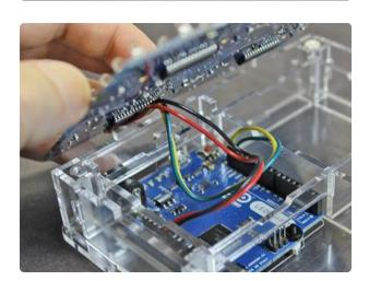
Now get the Trellis board ready. Remove the rubber buttons for the time being and turn the board face-down.
