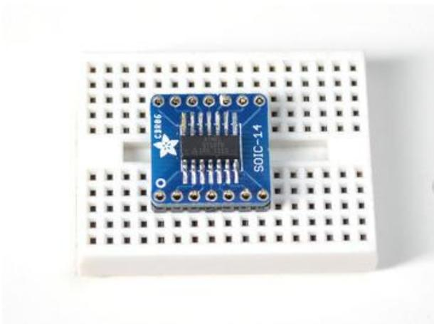
Break two pieces the same length as the pads on either side of the PCB and place them into a breadboard, long pins down. They should be parallel and the same distance as the PCB pads so that you can place the PCB on top with ease
