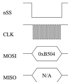
**Figure 12 Single Register Write to Initiate Self-Test**
