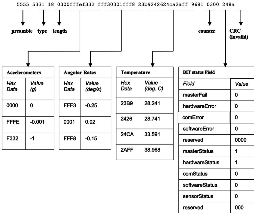
Figure 31 Example payload from Scaled Data Packet 1 (S1)
