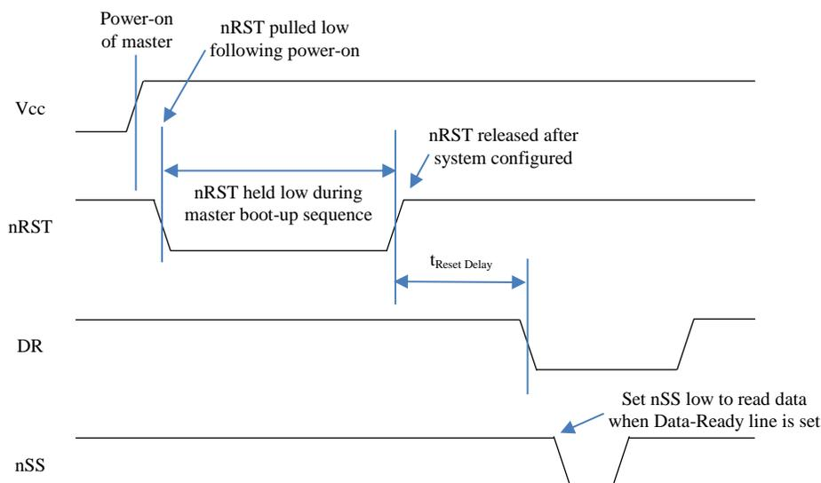
**Figure 15 Startup Timing**
