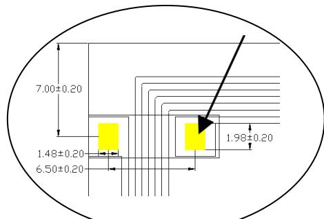
View from rear ferrite side, pads upward
