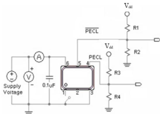
V<sub>dd</sub> = 3.3V: R<sub>1</sub>=R<sub>3</sub>=127Ω; R<sub>2</sub>=R<sub>4</sub>=82.5Ω
