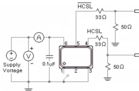
Note 9: Recommended test circuit images are representative of when the OE Function is located on Pin 1; when the OE Function is located on Pin 2, then Pin 1=No Connect & Pin 2=OE or No Connect.
