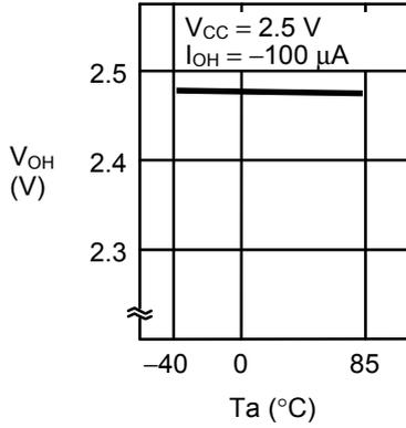
1. 20 High-level output voltage  $V_{OH}$
