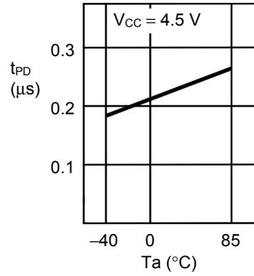
**2.7 Data output delay time  $t_{PD}$
