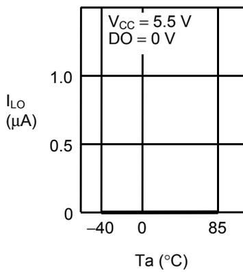
**1. 16 Output leakage current  $I_{LO}$
