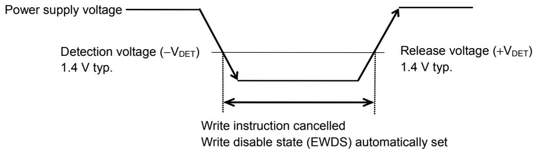
**Figure 12** Operation during Low Power Supply Voltage
