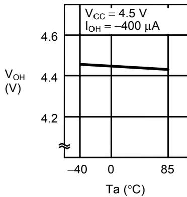
**1. 18 High-level output voltage  $V_{OH}$
