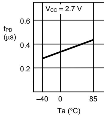
**2.8 Data output delay time  $t_{PD}$
