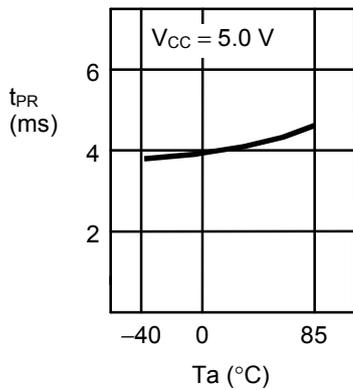
**2. 4 Write time  $t_{PR}$  vs. ambient temperature  $T_a$**
