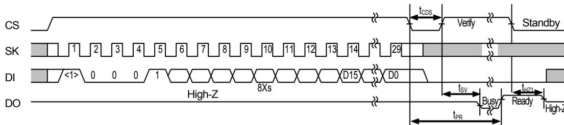
**Figure 9 Chip Write Timing**
