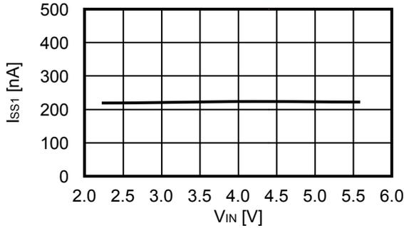
1.2 Current consumption during shutdown (I<sub>SSS</sub>) vs. Input voltage (V<sub>IN</sub>)
