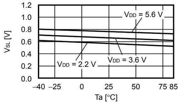
2. 16 UVLO detection voltage ( $V_{UVLO-}$ ) vs. Temperature ( $T_a$ )
