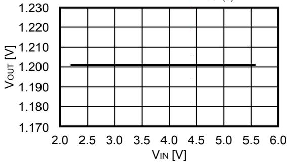
1.4 Output voltage (V<sub>OUT</sub>) vs. Input voltage (V<sub>IN</sub>)
