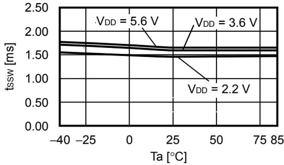
**2. 9 Soft-start time ( $t_{SS}$ ) vs. Temperature ( $T_a$ )**
