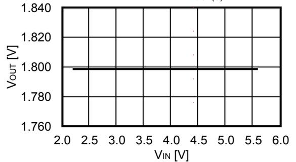
1.5 Output voltage (V<sub>OUT</sub>) vs. Input voltage (V<sub>IN</sub>)
