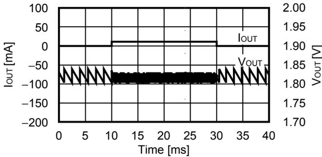
**3.4.2  $I_{OUT} = 0.1\text{ mA} \rightarrow 50\text{ mA} \rightarrow 0.1\text{ mA}$**
