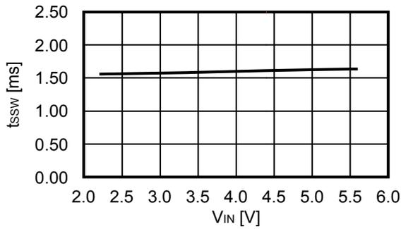
**1. 9 Soft-start time ( $t_{SS}$ ) vs. Input voltage ( $V_{IN}$ )**
