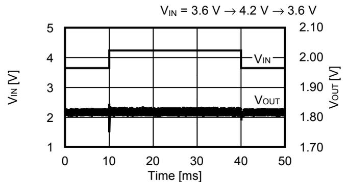
**3.4 Load fluctuation ( $V_{OUT} = 1.8\text{ V}$ ,  $V_{IN} = 3.6\text{ V}$ ,  $T_a = +25^\circ\text{C}$ )**
