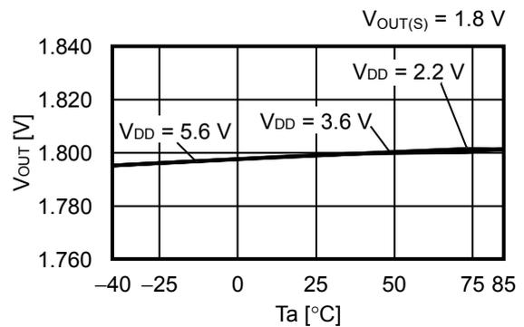
**2.5 Output voltage (VOUT) vs. Temperature (Ta)**
