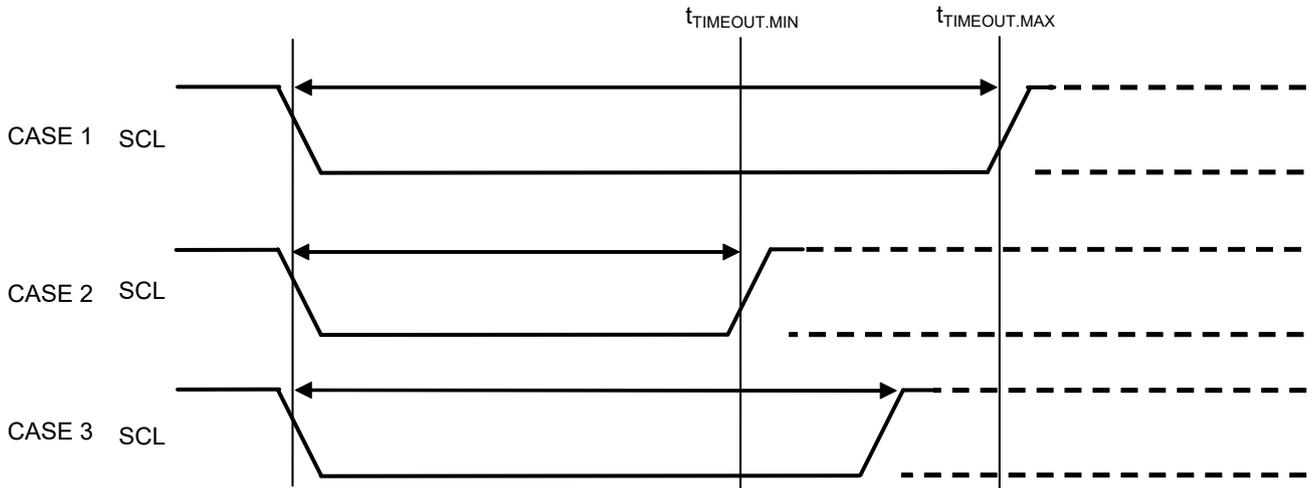
CASE1: SCL clock time "L" ( $t_{\text{LOW}} \geq t_{\text{TIMEOUT.MAX}}$ ), this IC will reset the bus communication and return to standby mode.
