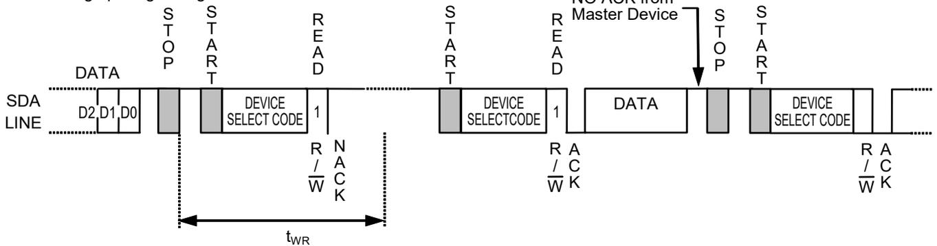
**Remark** Users are able to input data after acknowledge output in acknowledge polling during write. Users are able to read data after acknowledge output in acknowledge polling during read. However, after that users input the write instruction, a start condition may not be input during data output. Input a stop condition and the next instruction after acknowledge output and data output.
