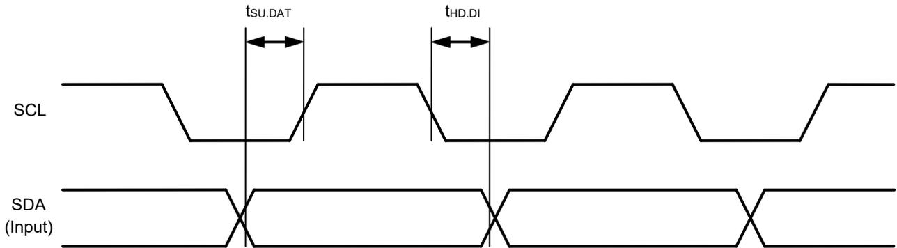
**Figure 5 Data Transmission Timing**
