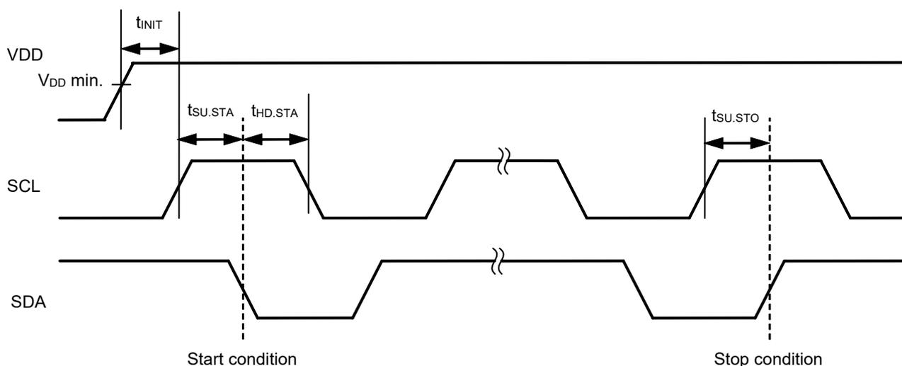
**Figure 4 Start / Stop Conditions after Power-on**
