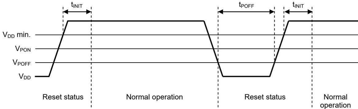
**Figure 15 Operation when Power Supply Voltage Drops and Power-on**
