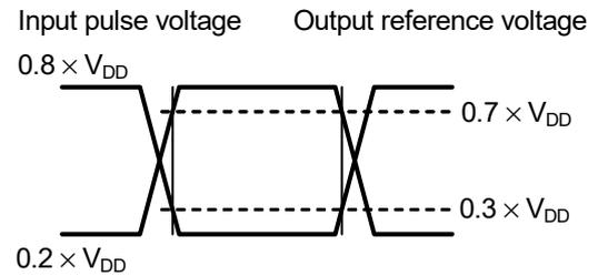
Figure 1 Input / Output Waveform during AC Measurement
