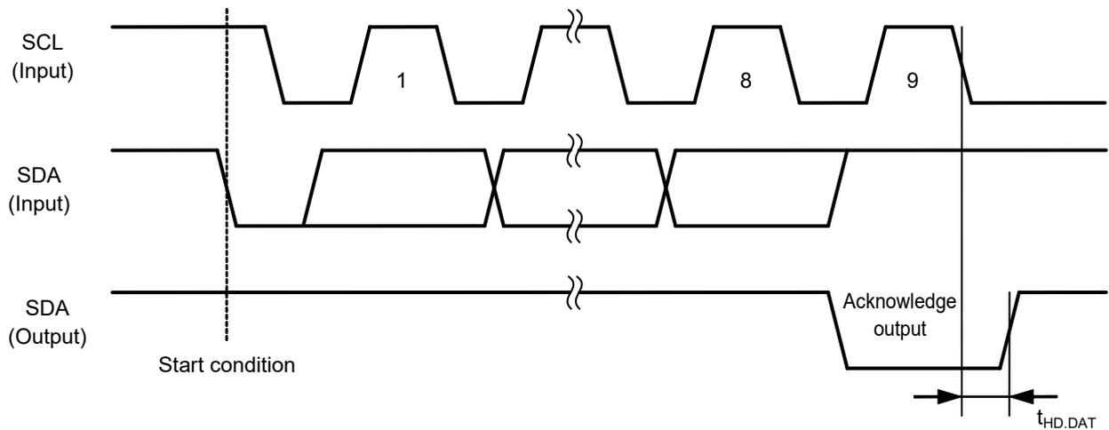
**Figure 6 Acknowledge Output Timing**
