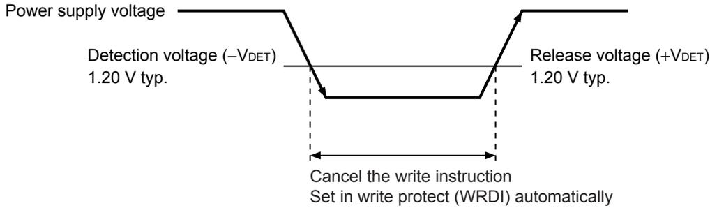
Figure 19 Operation during the Low Power Supply Voltage
