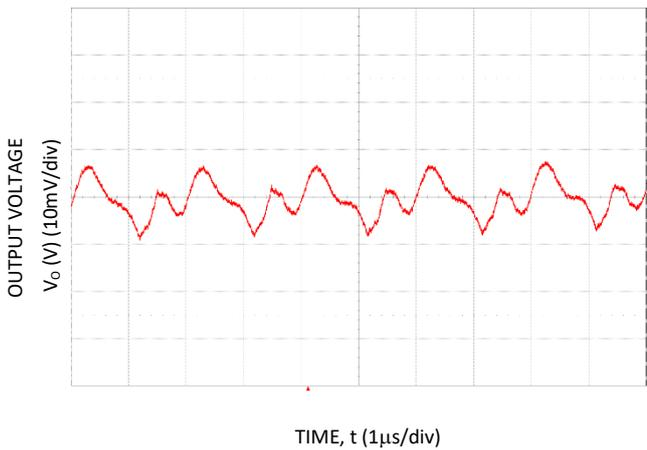
Figure 15. Typical output ripple and noise (C<sub>o</sub>=3X22µF ceramic, V<sub>IN</sub> = 12V, I<sub>o</sub> = I<sub>o,max</sub>).
