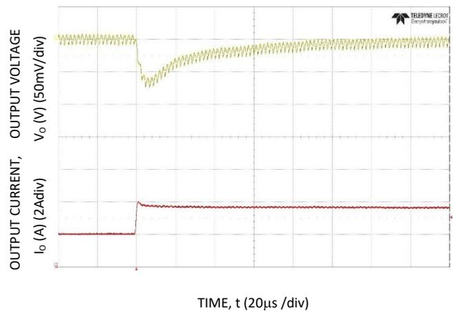
Figure 28. Transient Response to Dynamic Load Change from 50% to 100% at 12Vin, C<sub>out</sub>=3x47µF, C<sub>Tune</sub>=470pF, R<sub>Tune</sub>=300
