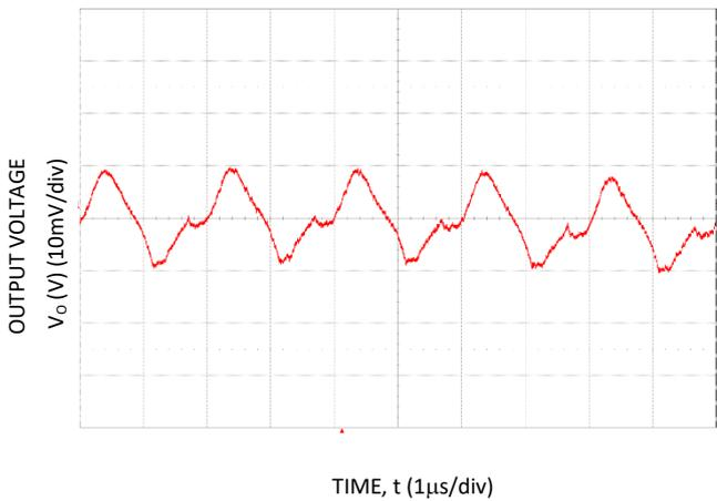
Figure 27. Typical output ripple and noise (C<sub>o</sub>=3x22µF ceramic, V<sub>IN</sub> = 12V, I<sub>o</sub> = I<sub>o,max</sub>).
