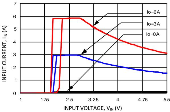
**Figure 7. Input voltage vs. Input Current**
