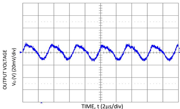
**Figure 9. Typical Output Ripple and Noise**
