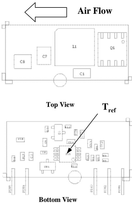
Figure 32. T<sub>ref</sub> Temperature measurement location.
