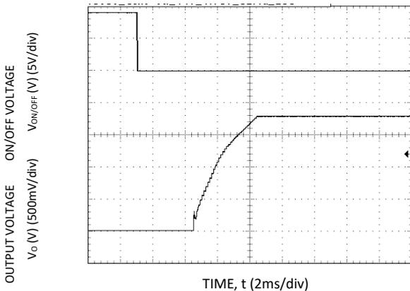
Figure 15. Typical Start-up Using On/Off Voltage ( $I_o = I_{o,max}$ ).
