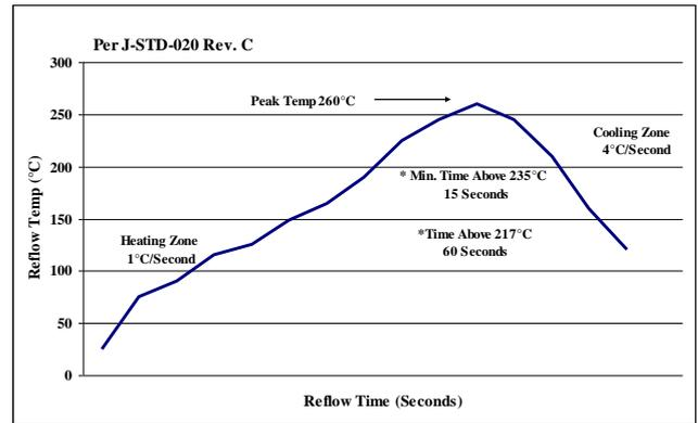
**NOTE:** Soldering outside of the recommended profile requires testing to verify results and performance.
