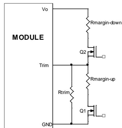
Figure 32. Circuit Configuration for margining Output voltage.
