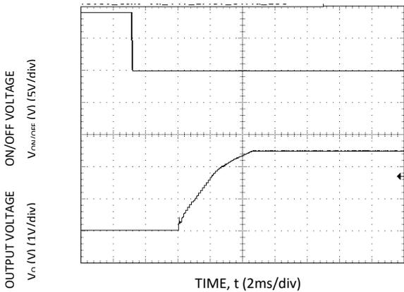
Figure 21. Typical Start-up Using On/Off Voltage ( $I_o = I_{o,max}$ ).
