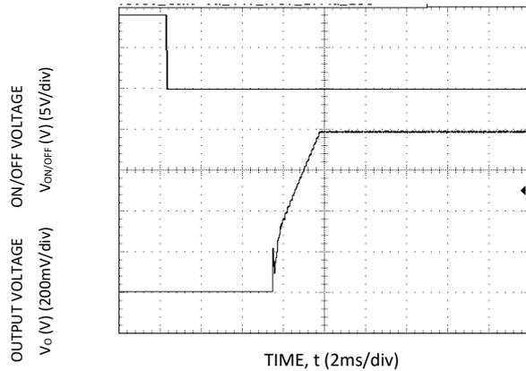
Figure 3. Typical Start-up Using On/Off Voltage ( $I_o = I_{o,max}$ ).
