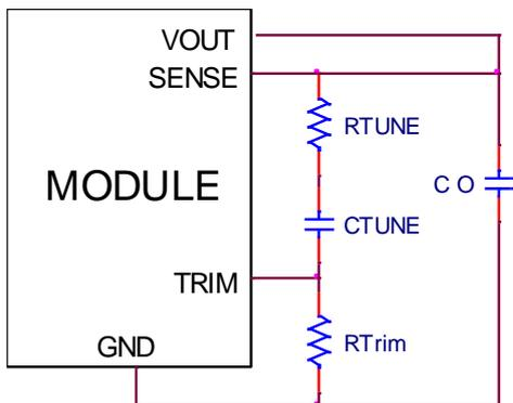
Figure 34. Circuit diagram showing connection of R<sub>TUNE</sub> and C<sub>TUNE</sub> to tune the control loop of the module.
