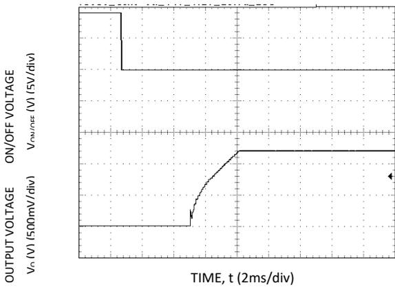
Figure 9. Typical Start-up Using On/Off Voltage ( $I_o = I_{o,max}$ ).
