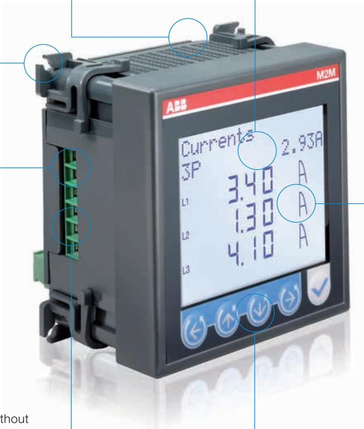
Multilingual backlit display with two lines of scrolling text to guide and help the user in reading data and programming. Safety password for protecting settings
